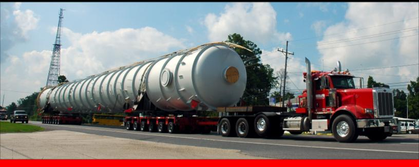
When a 250,000lb, 168' vessel needs to take a road trip, Berard's just the company to carry it. Covering over fifty miles of roads, city streets & highways, the vessel was successfully transported from the fabricators facility on two (2) six line THP platform trailers. One of the main goals was keeping the load level throughout the trip.
